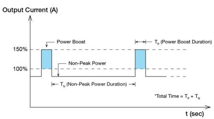
Fig. 3 Duty Cycle Calculation
