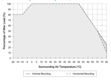
Fig. 1 De-rating for Vertical Mounting Orientation
