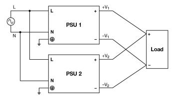
Fig. 5 **Parallel Operation Connection Diagram**
