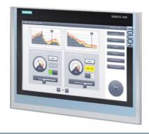
SIMATIC HMI TP1500 Comfort, Comfort Panel, touch operation, 15" widescreen TFT display, 16 million colors, PROFINET interface, MPI/PROFIBUS DP interface, 24 MB configuration memory, WEC 2013, configurable as of WinCC Comfort V14 SP1 with HSP, ambient temperature up to 50 °C (up to 55 °C with restrictions)
