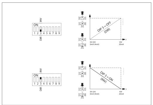
The actuator has a selection of DIP switches under the removable cover.
