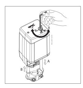
The manual override is applied by rotating the 4 mm Allen key (not supplied) to the required position. Observe the direction of the rotation symbol.
