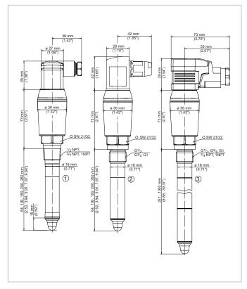
VEGAPOINT 23, standard version - thread, with valve plugs acc. to ISO 4400
