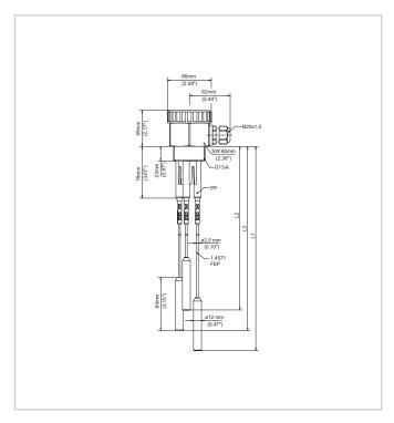
Conductive probe EL 6 L1-3*Probe length*
