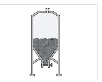
Level measurement in the building material silo
