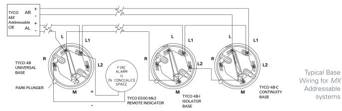
The MX CIE can be programmed to illuminate a Remote Indicator for detectors in alarm other than the detector base to which the Indicator is connected.
