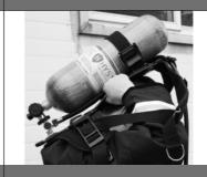
**4.**Put the apparatus overhead so that the shoulder strap is on the shoulder.
