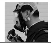
**13.**Connect the demand valve with the mask. Align the bayonet of the mask with the interface of the demand valve and press hard. The demand valve is securely connected with the mask when a "click" is heard
