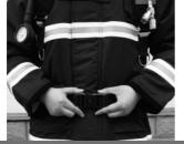
**5.**Insert the waistband buckle and adjust the waistband to a proper degree of tightness. Put on the assembled apparatus and adjust the harness to a proper position. Buckle up the waistband bayonet and adjust the length of the waistband to a proper position.
