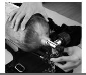
**1.**Lay the back plate harness assembly flat, confirm the integrity of O-ring on the pressure regulator valve, align the cylinder valve with the pressure regulator valve, and turn the pressure regulator wheel until the two valves are connected securely.
