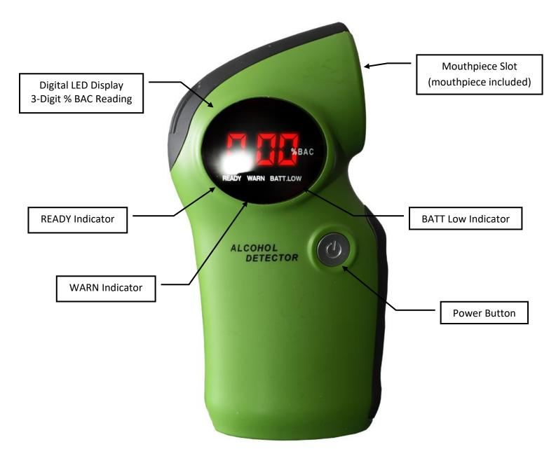
The AlcoMate Core (Model AL6000 Lite) analyzes a breath sample to detect alcohol in the lungs. This reading is then converted to blood alcohol concentration (BAC). The AlcoMate Core uses an advanced oxide semiconductor sensor to detect alcohol.
