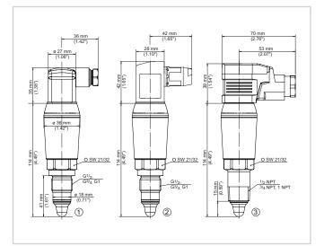
VEGAPOINT 31, standard version - thread with valve plugs acc. to ISO 4400
