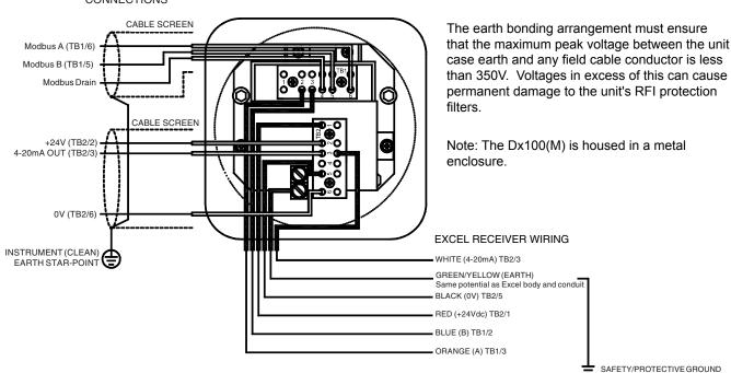
Where the DX 100(M) is not bonded to a local safety/protective earth then an external safety/protective earth needs to be made as shown.
