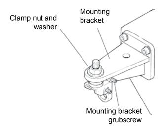
Do not fully tighten the nut (Refer to 3.73).
