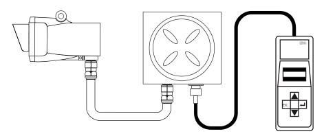
via another type of junction box, e.g. Honeywell Analytics Junction Box Part Number 00780-A-0100 - using the SHC Protection Device.
