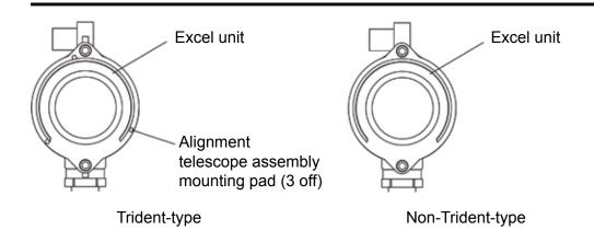
After deciding from the table which alignment telescope to use for the Excel units being aligned the telescope assembly must be fitted to each of the units in turn starting with the Transmitter. There are two ways of attaching the telescope to the Excel units - using latches or using a bayonet fitting. Depending on the type supplied refer to the relevant procedure described subsequently.
