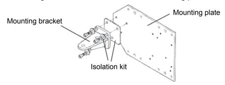
(3) Fit the mounting plate to the supporting structure.
