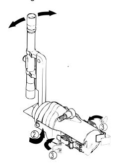
(d) Rotate the telescope to a comfortable viewing position, and then secure the latches as indicated by arrow 3.
