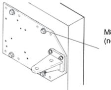
M8 mounting bolt - 4-off (not supplied) using **B** holes
