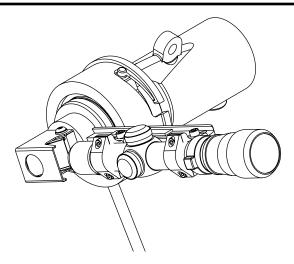
(d) With the other hand use the datum mount's locking handle to rotate the bayonet fitting in a clockwise direction until it is securely locked onto the cowl. The fitting is held tightly against the face of the cowl by means of hidden compression springs.
