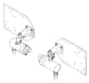
Ensure that the adjustment clamp's stub lever is approximately centrally positioned between the pivot block's grub screws. Adjust the screws if required.
