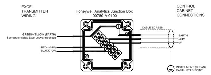
The earth bonding arrangement must ensure that the maximum peak voltage between the unit case earth and any field cable conductor is less than 350V. Voltages in excess of this can cause permanent damage to the unit's RFI protection filters.
