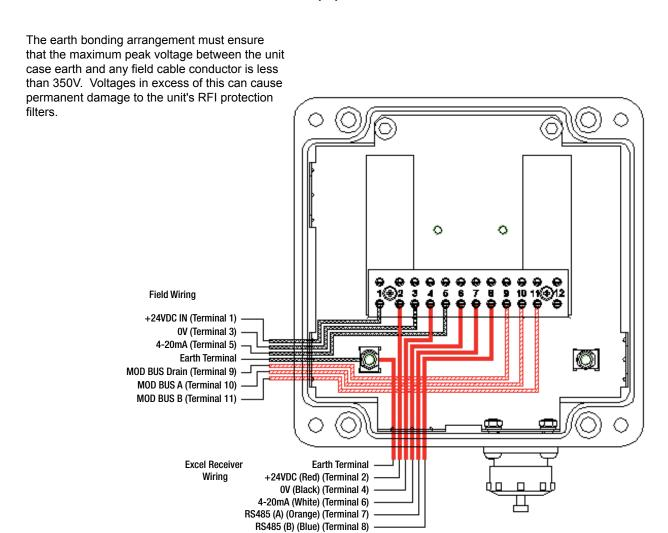
Note: Using metal cable glands may connect the armour of the cable to the Excel Body.
