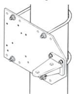
6in. U-bolt - 2-off (not supplied) using **B** holes
