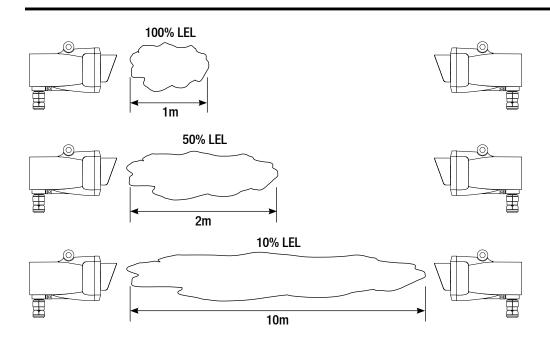
LEL.m monitoring is particularly beneficial while the Excel gas detector is protecting the perimeter of a plant or process, often reducing the quantity of point detectors required. The open path LEL.m system has the ability to detect leaks that point detectors may miss due to prevailing or changing wind directions, and can provide early warning of a dilute gas cloud when point detectors may not register any gas presence.
