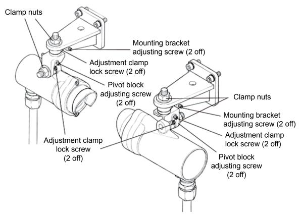
Initial coarse mechanical adjustment is first carried out by means of large clamping nuts and with the help of an alignment telescope.
