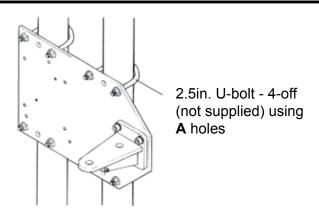
Mounting Plate Fixed to Twin Pipes/Poles
