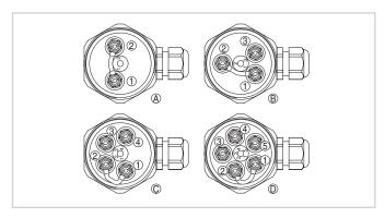
Connection compartment of the probe - 220  $k\Omega$  resistance between terminals 1 and 2
